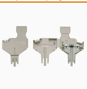
The component plug is used to integrate an electrical component in a disconnect terminal block. After soldering the electronic component, the plug can be integrated into the disconnection area of our disconnect terminal blocks and thus changes the disconnect terminal block into a modular terminal block with integrated electronic component.
