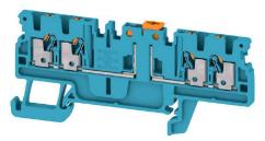
In some applications it makes sense to add a test point or a disconnect element to the feed through terminal for testing and safety purposes. With test disconnect terminals you measure electric circuits in the absence of voltage. While the disconnecting points clearance and creepage distance is not assessed in dimensional terms, the specified rated impulse voltage strength must be proven.
