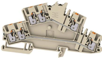
To feed through power, signal, and data is the classical requirement in electrical engineering and panel building. The insulating material, the connection system and the design of the terminal blocks are the differentiating features. A feed-through terminal block is suitable for joining and/or connecting one or more conductors. They could have one or more connection levels that are on the same potential or insulated against one another.
