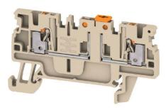
In some applications it makes sense to add a test point or a disconnect element to the feed through terminal for testing and safety purposes. With test disconnect terminals you measure electric circuits in the absence of voltage. While the disconnecting points clearance and creepage distance is not assessed in dimensional terms, the specified rated impulse voltage strength must be proven.
