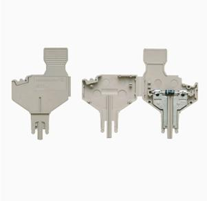
The component plug is used to integrate an electrical component in a disconnect terminal block. After soldering the electronic component, the plug can be integrated into the disconnection area of our disconnect terminal blocks and thus changes the disconnect terminal block into a modular terminal block with integrated electronic component.
