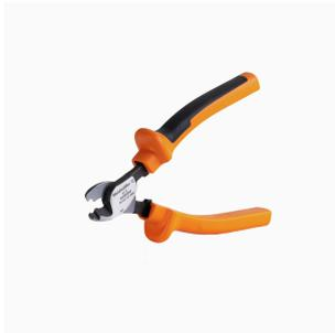
Cutting tools for conductors up to 8 mm, 12 mm, 14 mm and 22 mm outside diameter. The special blade geometry allows pinch-free cutting of copper and aluminium conductors with minimum physical effort. The cutting tools (KT 8 to KT 22) also come with VDE and GS-tested protective insulation up to 1,000 V in accordance with EN/IEC 60900.
