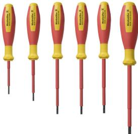
VDE insulated screwdriver sets, for working on live parts up to 1000 V AC and 1500 V DC, DIN EN 60900. IEC 900. Each piece is "GS" safety tested. Blade made from fully hardened, high-alloy chromium-vanadium-molybdenum steel, gun-metal finish.
