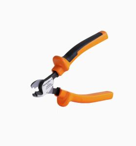
Cutting tools for conductors up to 8 mm, 12 mm, 14 mm and 22 mm outside diameter. The special blade geometry allows pinch-free cutting of copper and aluminium conductors with minimum physical effort. The cutting tools (KT 8 to KT 22) also come with VDE and GS-tested protective insulation up to 1,000 V in accordance with EN/IEC 60900.
