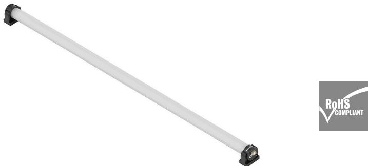
The E-series, with standard and premium lights, is ideal for focused lighting in work areas. Swiveling mounting brackets provide the necessary flexibility in the positioning of the lighting field. Thanks to the built-in M8 connectors, a simple and quick connection is given and allows the connection of several lights. The cover made of robust PMMA not only provides the necessary protection (IP54) but also ensures a homogeneous illumination with 5.700K.
