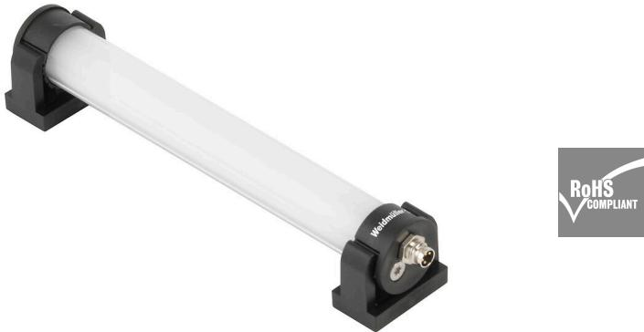
The E-series, with standard and premium lights, is ideal for focused lighting in work areas. Swiveling mounting brackets provide the necessary flexibility in the positioning of the lighting field. Thanks to the built-in M8 connectors, a simple and quick connection is given and allows the connection of several lights. The cover made of robust PMMA not only provides the necessary protection (IP54) but also ensures a homogeneous illumination with 5.700K.
