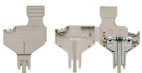
The component plug is used to integrate an electrical component in a disconnect terminal block. After soldering the electronic component, the plug can be integrated into the disconnection area of our disconnect terminal blocks and thus changes the disconnect terminal block into a modular terminal block with integrated electronic component.
