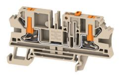
In some applications it makes sense to add a test point or a disconnect element to the feed through terminal for testing and safety purposes. With test disconnect terminals you measure electric circuits in the absence of voltage. While the disconnecting points clearance and creepage distance is not assessed in dimensional terms, the specified rated impulse voltage strength must be proven.
