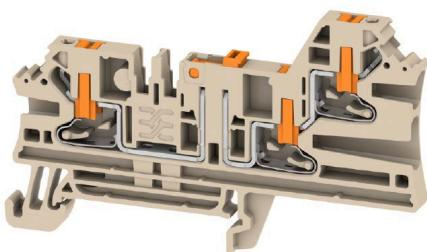
In some applications it makes sense to add a test point or a disconnect element to the feed through terminal for testing and safety purposes. With test disconnect terminals you measure electric circuits in the absence of voltage. While the disconnecting points clearance and creepage distance is not assessed in dimensional terms, the specified rated impulse voltage strength must be proven.
