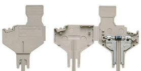
The component plug is used to integrate an electrical component in a disconnect terminal block. After soldering the electronic component, the plug can be integrated into the disconnection area of our disconnect terminal blocks and thus changes the disconnect terminal block into a modular terminal block with integrated electronic component.
