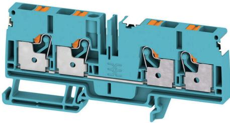
To feed through power, signal, and data is the classical requirement in electrical engineering and panel building. The insulating material, the connection system and the design of the terminal blocks are the differentiating features. A feed-through terminal block is suitable for joining and/or connecting one or more conductors. They could have one or more connection levels that are on the same potential or insulated against one another.
