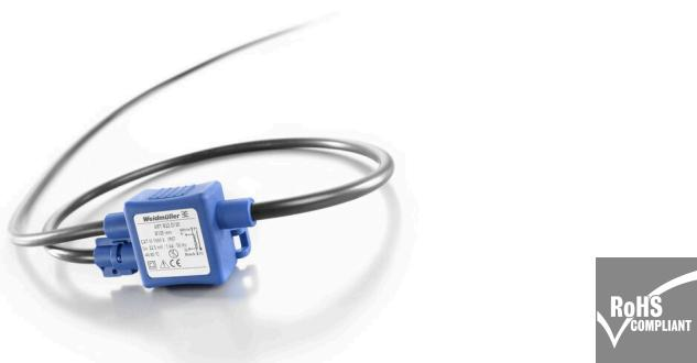
**Rogowski coil** A Rogowski coil is a closed air coil without a ferromagnetic core used for floating potential measurement of AC and pulse currents. Measurement with the Rogowski coil is used widely in technology, as it can be retroactively integrated without separating the primary electric circuit in existing systems. Because this method shows no saturation effect, even the smallest currents and high-frequency harmonics can be measured without loss of accuracy.
