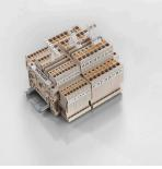
SnapMark - this tag carrier has been developed especifically for the I-series double-level terminal IDK 1.5N. The flexible pivot mechanism allows cross-connections to be easily installed or removed. It can hold four DEK 5 labelling tags or two WS 10/5 Middle connector markers.
