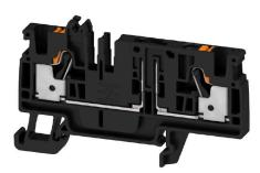
In some applications it is useful to protect the feed through connection with a separate fuse. Fuse terminal blocks are made up of one terminal block bottom section with a fuse insertion carrier. The fuses vary from pivoting fuse levers and pluggable fuse holders to screwable closures and flat plug-in fuses.
