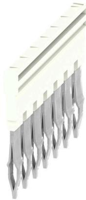
The distribution or multiplication of a potential to adjoining terminal blocks is realized via a cross-connection. Additional wiring effort can be easily avoided. Even if the poles are broken out, contact reliability in the terminal blocks is still ensured. Our portfolio offers pluggable and screwable cross-connection systems for modular terminal blocks.
