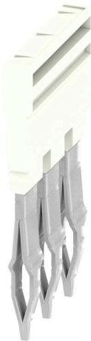
The distribution or multiplication of a potential to adjoining terminal blocks is realized via a cross-connection. Additional wiring effort can be easily avoided. Even if the poles are broken out, contact reliability in the terminal blocks is still ensured. Our portfolio offers pluggable and screwable cross-connection systems for modular terminal blocks.
