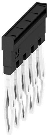
The distribution or multiplication of a potential to adjoining terminal blocks is realized via a cross-connection. Additional wiring effort can be easily avoided. Even if the poles are broken out, contact reliability in the terminal blocks is still ensured. Our portfolio offers pluggable and screwable cross-connection systems for modular terminal blocks.
