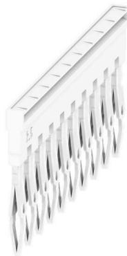
The distribution or multiplication of a potential to adjoining terminal blocks is realized via a cross-connection. Additional wiring effort can be easily avoided. Even if the poles are broken out, contact reliability in the terminal blocks is still ensured. Our portfolio offers pluggable and screwable cross-connection systems for modular terminal blocks.
