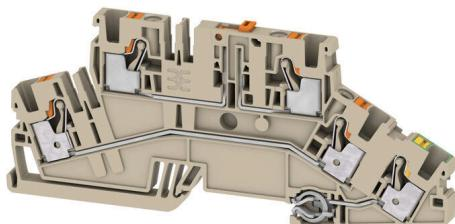
In some applications it makes sense to add a test point or a disconnect element to the feed through terminal for testing and safety purposes. With test disconnect terminals you measure electric circuits in the absence of voltage. While the disconnecting points clearance and creepage distance is not assessed in dimensional terms, the specified rated impulse voltage strength must be proven.
