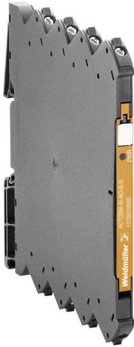
The universal frequency measuring transducer, which can be configured via software, disconnects and converts input signals (frequency, Namur, NPN, PNP, speedometer, TTL and S0) into an active analogue standard output signal. The power supply is galvanically isolated from the input and output (3-way isolation) by means of direct wiring. The model ACT20M-FRQ-AO-S can be supplied via the Weidmüller DIN rail bus
