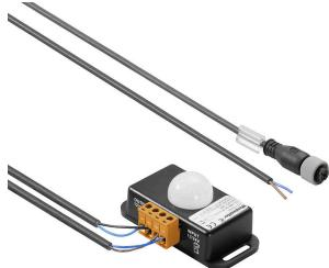
Motion detector for the WIL-LED luminaire with screw connection, 3m supply cable and M12 cable for connection to the WIL lamp. Switching time adjustable.
