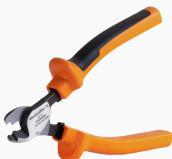
Cutting tools for conductors up to 8 mm, 12 mm, 14 mm and 22 mm outside diameter. The special blade geometry allows pinch-free cutting of copper and aluminium conductors with minimum physical effort. The cutting tools (KT 8 to KT 22) also come with VDE and GS-tested protective insulation up to 1,000 V in accordance with EN/IEC 60900.
