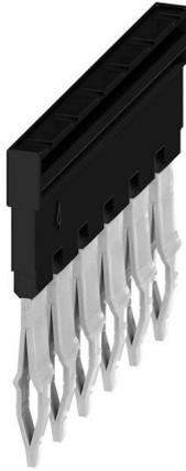
The distribution or multiplication of a potential to adjoining terminal blocks is realized via a cross-connection. Additional wiring effort can be easily avoided. Even if the poles are broken out, contact reliability in the terminal blocks is still ensured. Our portfolio offers pluggable and screwable cross-connection systems for modular terminal blocks.
