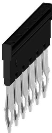
The distribution or multiplication of a potential to adjoining terminal blocks is realized via a cross-connection. Additional wiring effort can be easily avoided. Even if the poles are broken out, contact reliability in the terminal blocks is still ensured. Our portfolio offers pluggable and screwable cross-connection systems for modular terminal blocks.
