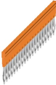
The distribution or multiplication of a potential to adjoining terminal blocks is realized via a cross-connection. Additional wiring effort can be easily avoided. Even if the poles are broken out, contact reliability in the terminal blocks is still ensured. Our portfolio offers pluggable and screwable cross-connection systems for modular terminal blocks.
