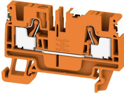
To feed through power, signal, and data is the classical requirement in electrical engineering and panel building. The insulating material, the connection system and the design of the terminal blocks are the differentiating features. A feed-through terminal block is suitable for joining and/or connecting one or more conductors. They could have one or more connection levels that are on the same potential or insulated against one another.
