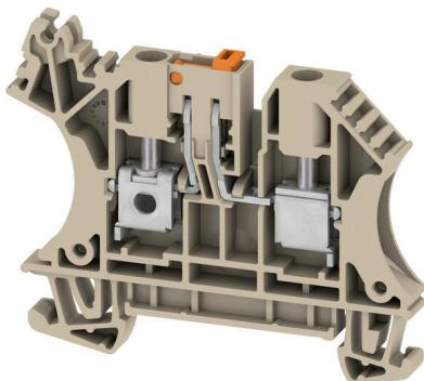
In some applications it makes sense to add a test point or a disconnect element to the feed through terminal for testing and safety purposes. With test disconnect terminals you measure electric circuits in the absence of voltage. While the disconnecting points clearance and creepage distance is not assessed in dimensional terms, the specified rated impulse voltage strength must be proven.
