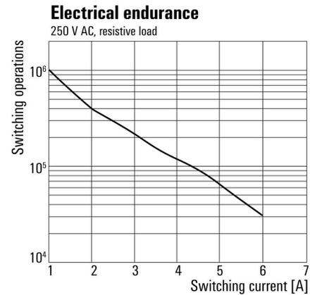
Electrical service life 230 V AC resistive load
