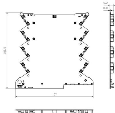
Base element without cut-out in snap-in foot area
