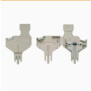
The component plug is used to integrate an electrical component in a disconnect terminal block. After soldering the electronic component, the plug can be integrated into the disconnection area of our disconnect terminal blocks and thus changes the disconnect terminal block into a modular terminal block with integrated electronic component.
