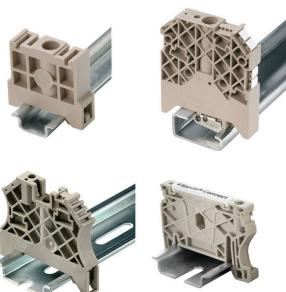
Weidmüller's range of products includes end brackets that guarantee a permanent, reliable mounting on the terminal rail and prevent sliding. Versions with and without screws are available. The end brackets include marking options, also for group markers, and also a test plug holder.
