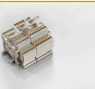
SnapMark - this tag carrier has been developed specifically for the I-series double-level terminal IDK 1.5N. The flexible pivot mechanism allows cross-connections to be easily installed or removed. It can hold four DEK 5 labelling tags or two WS 10/5 Middle connector markers.
