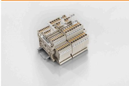
SnapMark - this tag carrier has been developed specifically for the I-series double-level terminal IDK 1.5N. The flexible pivot mechanism allows cross-connections to be easily installed or removed. It can hold four DEK 5 labelling tags or two WS 10/5 Middle connector markers.
