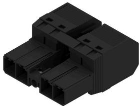
180° inverted inverse voltage-safe male header with PUSH IN connection technology for field wiring. With automatically locking middle flange for field wiring in 6 mm<sup>2</sup> with 7.62 pitch. Also ideal as a touch-safe solution for inverse voltages. Meets the requirements of UL 1059 600 V class C and IEC 61800-5-1. On request, also available without middle flange.
