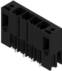
Single-row, high-performance male header for side-by-side mounting without sacrificing any poles or with patented flange for fast fixing without tools. Maximum connection and operating reliability thanks to a mating profile that prevents incorrect connection, with unique coding diversity and additional fastening in the flange. 3.5 mm pin length is optimised for lead-free wave soldering.
