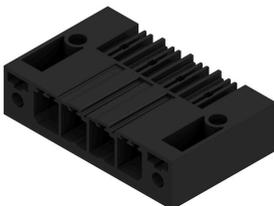
Single-row, high-current and high-performance male headers for side-by-side mounting without sacrificing any poles or with flange for fast fixing without tools. Maximum connection and operating reliability thanks to a mating profile that prevents incorrect connection, unique coding diversity and additional fastening in the flange.
