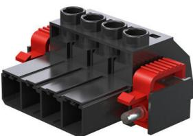
High-performance male header with the proven, 100% maintenance-free Weidmüller steel clamping yoke. Side-by-side mounting without sacrificing any poles or with patented multifunction flange for secure, fast fixing without tools. Maximum connection and operating reliability thanks to a mating profile that prevents incorrect connection, unique coding diversity, incorrect wiring protection. Suitable for labelling.
