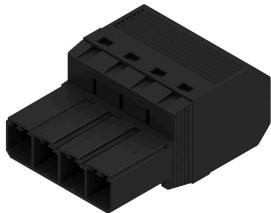
180° inverted pin header with PUSH IN connection technology for field wiring in 6mm<sup>2</sup> in a 7.62 pitch, as a "three-flange variant" for enclosure feed-through. Suitable for enclosures with a max. wall thickness of 2mm. Also perfect as a touch-safe solution for reverse voltages. Meets the requirements of UL1059 600 V Class C and IEC 61800-5-1.
