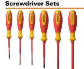
VDE insulated screwdriver sets, for working on live parts up to 1000 V AC and 1500 V DC, DIN EN 60900. IEC 900. Each piece is "GS" safety tested. Blade made from fully hardened, high-alloy chromium-vanadium-molybdenum steel, gun-metal finish.
