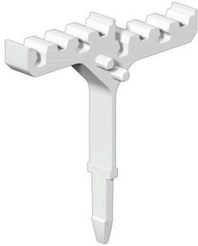
SnapMark - this tag carrier has been developed specifically for the I-series double-level terminal IDK 1.5N. The flexible pivot mechanism allows cross-connections to be easily installed or removed. It can hold four DEK 5 labelling tags or two WS 10/5 Middle connector markers.
