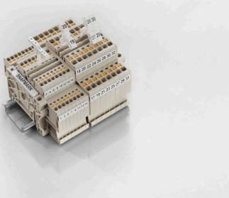
SnapMark - this tag carrier has been developed especially for the I-series double-level terminal IDK 1.5N. The flexible pivot mechanism allows cross-connections to be easily installed or removed. It can hold four DEK 5 labelling tags or two WS 10/5 Middle connector markers.
