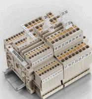
SnapMark - this tag carrier has been developed specifically for the I-series double-level terminal IDK 1.5N. The flexible pivot mechanism allows cross-connections to be easily installed or removed. It can hold four DEK 5 labelling tags or two WS 10/5 Middle connector markers.
