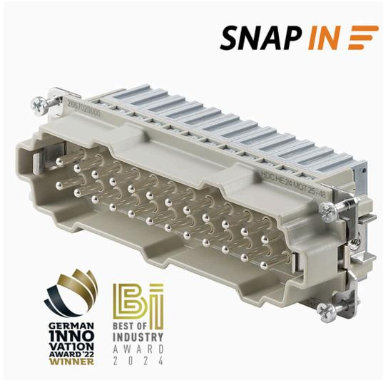
With the SNAP IN connection, the conductor connection level is already open and the stripped connector can be simply inserted. In the end position, the patented clamping mechanism closes automatically. As a result, it requires virtually no maintenance and a safe, permanent and vibration-proof connection is established. Weidmüller is therefore the first and only manufacturer to offer this innovative connection system.
