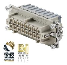
With the SNAP IN connection, the conductor connection level is already open and the stripped connector can be simply inserted. In the end position, the patented clamping mechanism closes automatically. As a result, it requires virtually no maintenance and a safe, permanent and vibration-proof connection is established. Weidmüller is therefore the first and only manufacturer to offer this innovative connection system.
