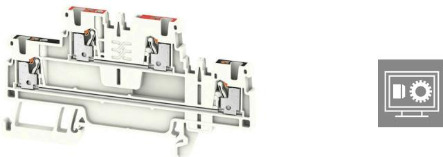
The Klippon® Connect KNX-terminal blocks provide the wiring of the main and reserve leads for KNX Bus wiring systems within a 7 mm combined block width. At each level, a double cross-connection point yields quick and easy distribution of the potential within the terminal.
