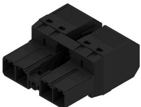
180° inverted inverse voltage-safe male header with PUSH IN connection technology for field wiring. With automatically locking middle flange for field wiring in 6 mm<sup>2</sup> with 7.62 pitch. Also ideal as a touch-safe solution for inverse voltages. Meets the requirements of UL1059 600 V class C and IEC 61800-5-1. On request, also available without middle flange.
