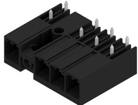
270° male header with middle flange with a 7.62 pitch. Meets the requirements of IEC 61800-5-1 and enables UL approval as per UL840 600 V. Without a female header, the mating profile guarantees minimum touch safety of >3 mm with 20 N pressure on the test finger. The automatically locking middle flange which can optionally also be screwed, reduces space requirements by one pitch width in comparison with conventional solutions.
