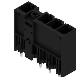
180° male header with middle flange with a 7.62 pitch. Meets the requirements of IEC 61800-5-1 and enables UL approval as per UL840 600 V. Without a female header, the mating profile guarantees minimum touch safety of >3 mm with 20 N pressure on the test finger. The automatically locking middle flange which can optionally also be screwed, reduces space requirements by one pitch width in comparison with conventional solutions.
