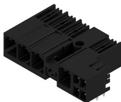
Combined 90° male header with power and signal contacts in PUSH IN connection technology incl. self-locking middle flange interlock and (optional) pluggable shield connection with a 7.62 pitch.
