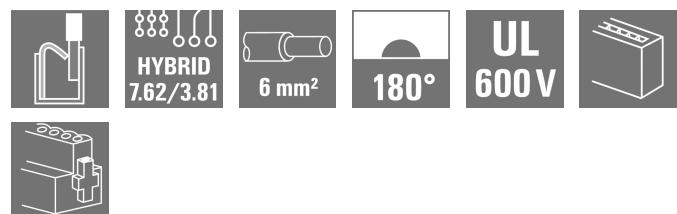
180° female plug with energy and signal contacts in PUSH IN wire connection in 7.62 pitch.
