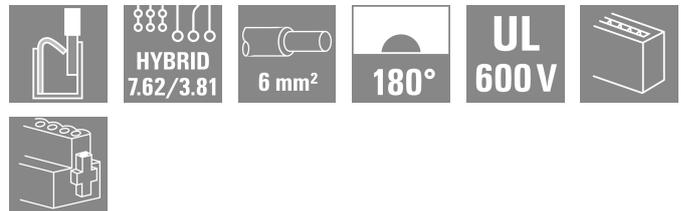
180° female plug with energy and signal contacts in PUSH IN wire connection in 7.62 pitch. Fulfils the IEC 61800-5-1 requirement and for the energy contact UL 1059 ClassC 600 V. The self-locking middle flange with automatic interlock reduces the space requirements by one pitch width in comparison with conventional solutions. Optionally also available with additional mounting screw.
